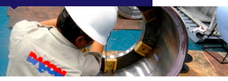
UT uses high frequency ultrasonic waves to detect surface breaking and internal imperfections, measure material thickness and determine acceptance or rejection of a test object based on a reference code or standard. Flaw detection is a fast and accurate inspection method to evaluate internal product integrity.
