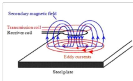
**Figure 2:** eddy currents generate secondary magnetic field in the receiver coil
