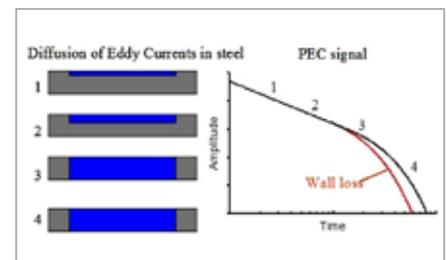
**Figure 3:** Diffusion of eddy currents. The onset of fast decay occurs when the far surface is reached
