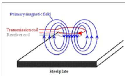
**Figure 1:** Magnetization of the steel
