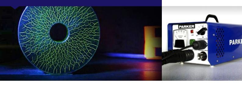
The Dacon used Parker Research DA-1500 portable heavy duty magnetic inspection unit provides high output AC or HWDC fields for magnetic particle inspection.
