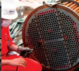
MFL is a technique used for the inspection of tubes made of ferrous materials. This technique will normally be applied as a fast screening technique if small diameter pitting is expected. Because of limitations to its sizing abilities the technique is not often used as a stand—alone technique.
