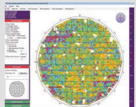
MFLi VIEW 'Intensity' view of MFL data. Used to classify and evaluate defects.
