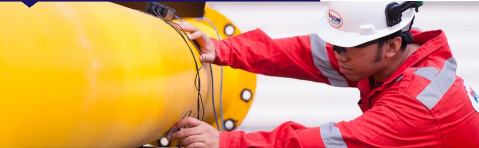
Flooded Member Detection is generally used to verify if the presence of and fill level of a liquid inside a pipe section. The FMD tool can also be used to verify the location of any dense (solid) material inside a pipe section.
