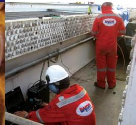
Eddy Current is notably the fastest and most preferred tube inspection technique available. Eddy Current however can only be used on non-ferrous materials like Brass, Copper, Copper-Nickel and Stainless steel.
