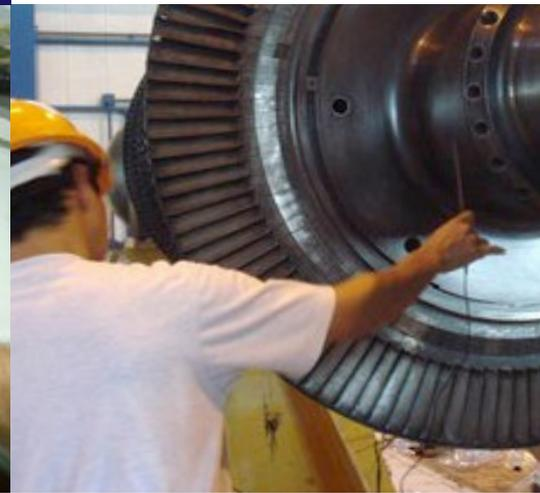
In order to perform Magnetic Particle Test, it is necessary for the ferromagnetic test specimen to be magnetized.
