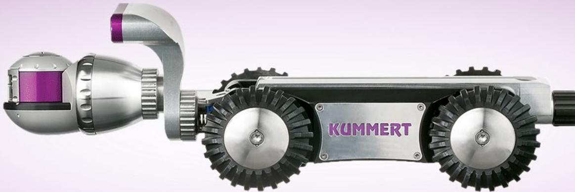
This RVI tool is a high resolution camera head with pan/tilt capability attached to a 4 wheel drive crawler pulling a 260 meter long Kevlar reinforced cable, capable of entering nozzles, pipes and passages with diameter from 130 mm upwards. Its extended length of 260 meter allows the crawler to be driven or dropped into a tank or pipeline to view in clear detail the internal condition.
